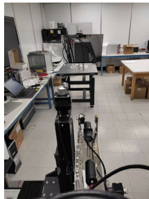
(b) Point-like reflected spot size measurement station.
