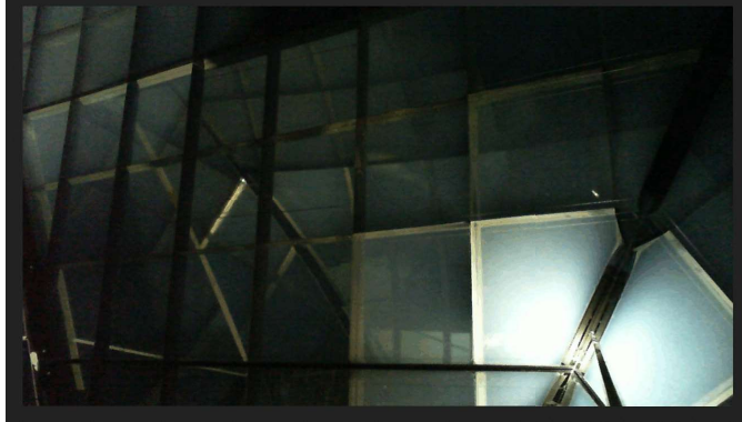
Figure 2.17: View of the aerogel inside the RICH after its installation in Hall B.
