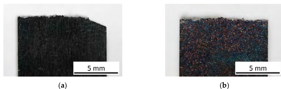
Figure 7. Representative stereomicroscope images of the fracture profiles of the (a) V-notched and (b) unnotched samples.
