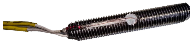
FIGURE 5.11: Stud bolt with strain gauges installed.
