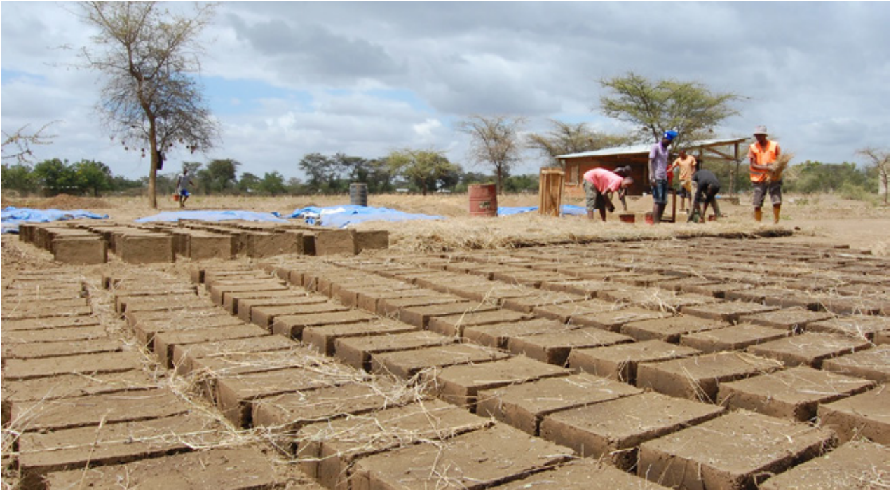
6.5 Sun-dried or adobe bricks laying on the floor to dry after production. Source: Own picture
