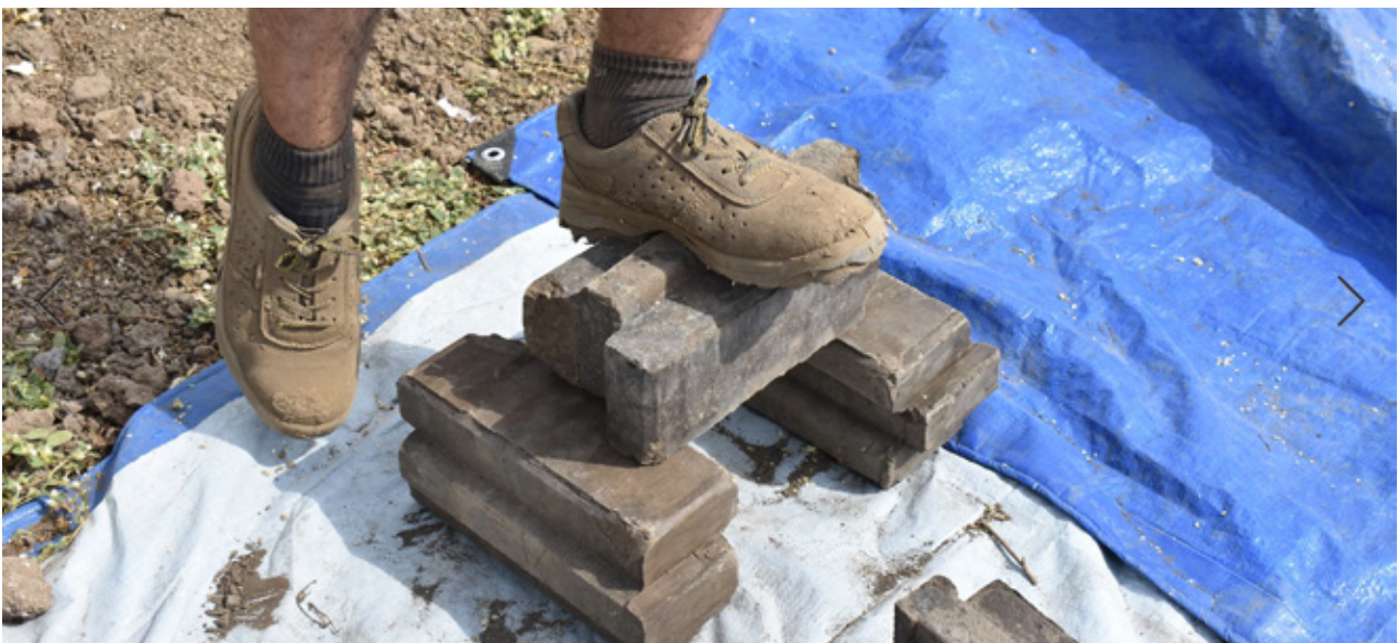
8.3 Testing the strength of the interlocking compressed bricks.
