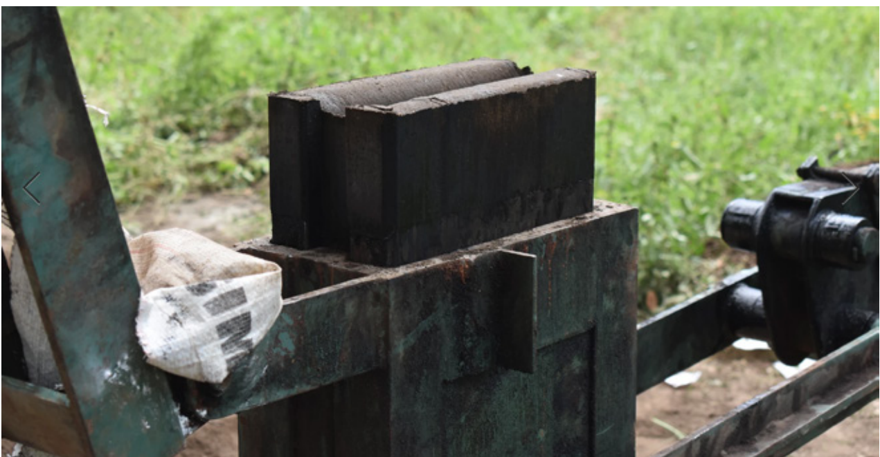
6.21 Compressing machine and CSEB just manufactured in Maji Moto. Source: C-re-aid website
