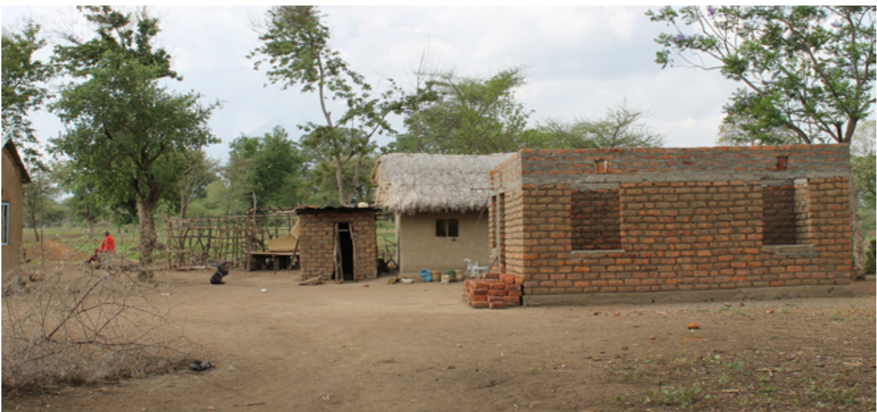
5.4 Mud house with thatched roof on the back and new house built with burnt bricks on the front in Maji Moto. Source: Own picture
