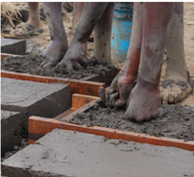
3.13 Adobe bricks being produced with mud and straw. Source: C-re-aid Website
