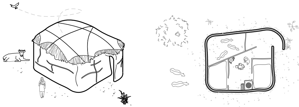
14.6 Floor plan and axonometric view of the indigenous Maasai hut, which usually lacks windows and doors. Own illustration
