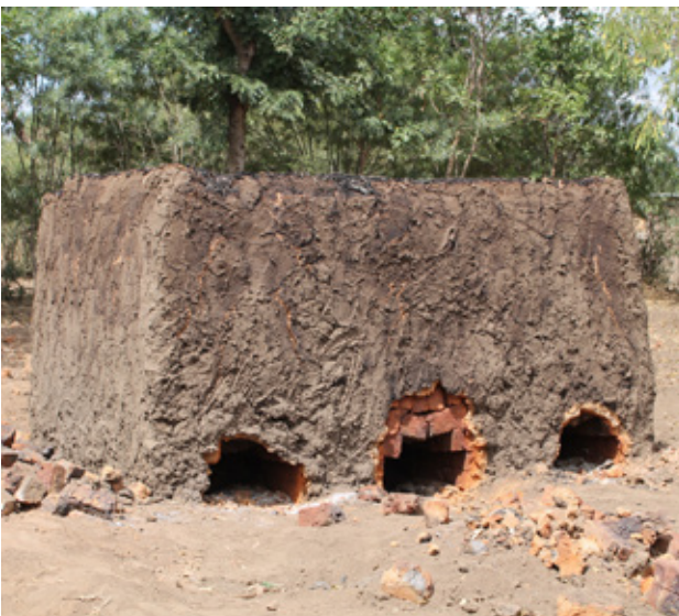
3.15 Hand-made oven with ready fired bricks inside. The surface has been covered with mud and cow dung. Source: Own picture
