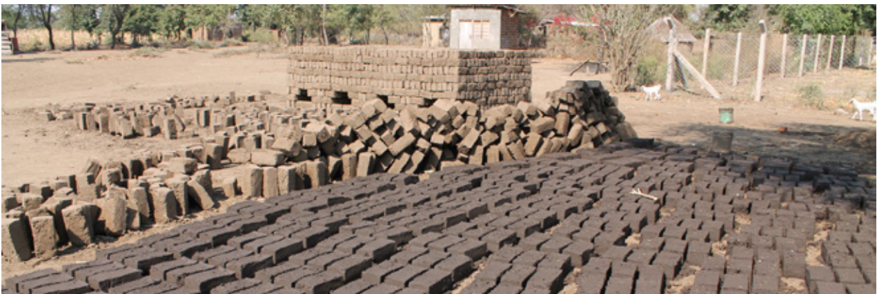
6.6 The three phases of producing fired bricks: moulded, drying and piled to be fired. Source: Own picture
