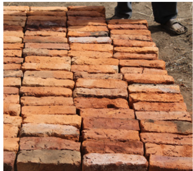
3.16 Fired bricks after baking 48 hours. These are ready to be used in construction. Source: Own picture
