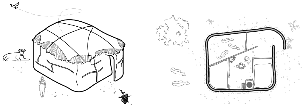
3.5 Axonometric view and floor plan of a typical indigenous Enkaji. Walls are built with the wattle & daub technique and thatched roof. Own illustration.
