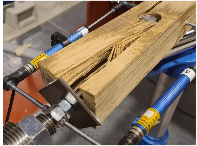
Fig. 12. Failure modes observed at the end of cyclic pull-pull tests (class 12.9 connectors): (a) specimen B-50-12.9-CO-100-1; (b) specimen B-50-12.9-CO-150-2.
