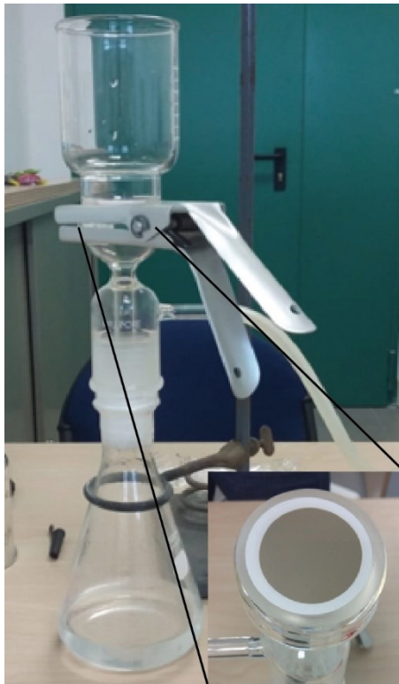
Figure 3.3: Millipore filtration apparatus, with detail of the thin film of clays deposited on the filter.
