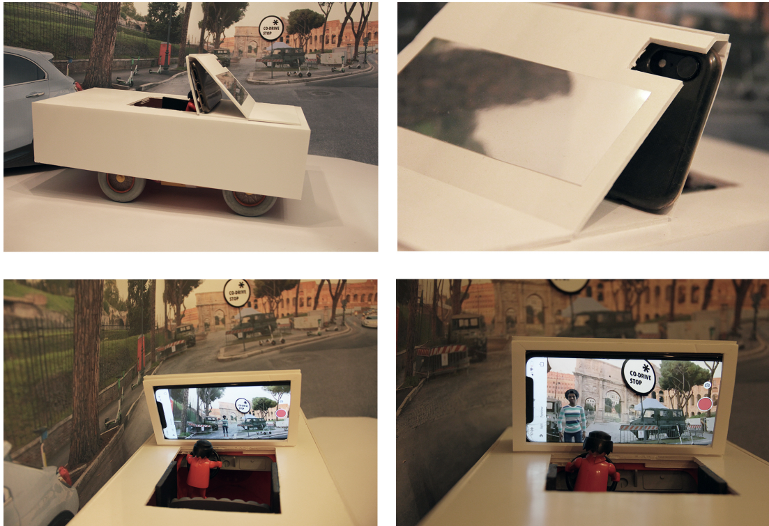
Figure 5.1: The AR diorama is composed by a model car and an Iphone whose display works as AR enabled windshield.
