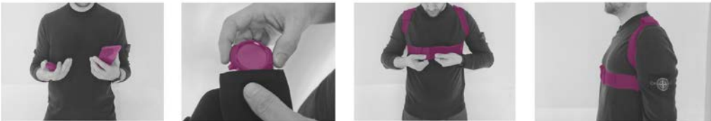
Fig. 3 PASSO, wearing the device. The final prototype is a sort of postural band for the upper part of the body, allowing the positioning of the SW face in several configurations depending on personal preferences and medical needs. Credits: Silvia Imbesi.
