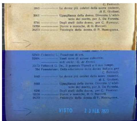
Fluorescent ink (commercially available) applied on paper under normal (top) and UV light (bottom)
