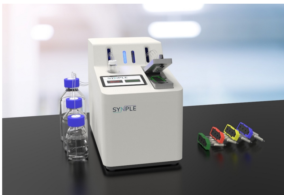
Figure 5.1: Synple Chem console and reagent cartridges (image adapted from: https://synplechem.com/images/2021/05/12/machinev_wlines.38_hp.jpg , 19/11/2022).
