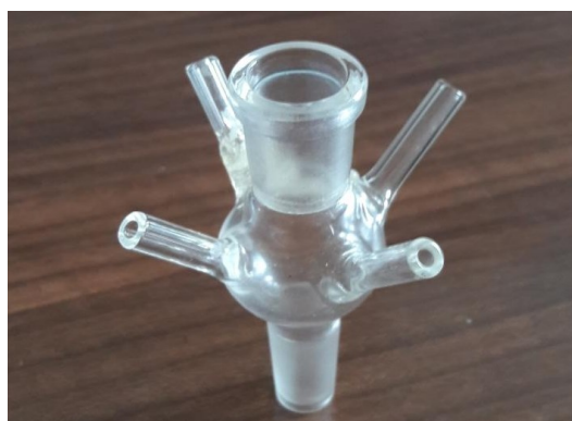
Fig.30 Image of the six-ways connector located on the top of the cell
