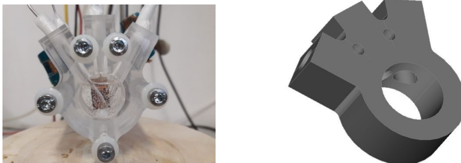
Fig.18 On the left type 2 electrochemical cell for the accumulation and analysis of water soluble products (formate and alcohols); on the right is shown a 3D rendering of one of the modular components
