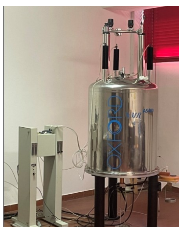
Fig.24 Varian Mercury Plus model at University of Ferrara (on the left) and 1 H 1D NMR spectrum on a sample of 0.5 M KHCO 3 containing a mixture of products (on the right)
