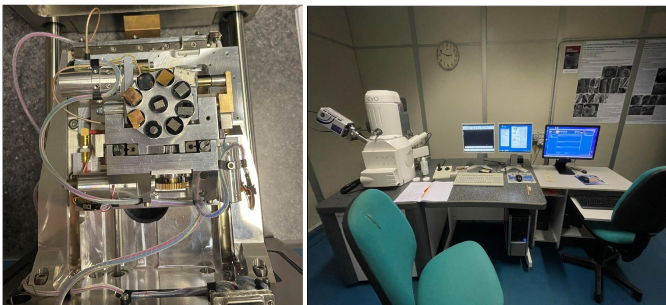
Fig.23 On the left the sample holder of the electron scanning microscope is shown; on the right the general set up of the instrument.
