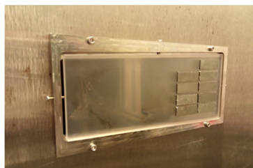
Fig. 7. Left: Laue lens module with nine crystals glued on top. The steel frame supporting the glass substrate is visible. Right: Misalignment of the crystals vs time from bonding.
