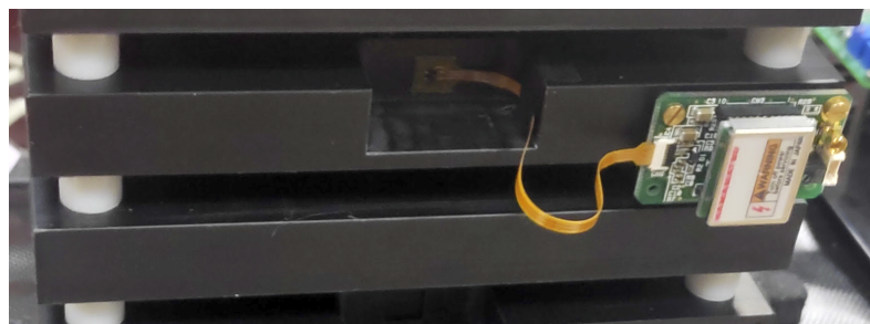
Figure 5. Close-up of the Hamamatsu 1663 SiPM (Hamamatsu Photonics K.K., Shizuoka, Japan) module located on the detector tower. In the center of the picture, connected with a kapton flex cable, is the SiPM ( 3 \times 3 \text{ mm}^2 ) and the temperature sensor. The electronic unit, containing the power supply, the temperature compensation circuit, and the pre-amplification stage, is located on the right of the picture. The size of the electronic unit is 36 \times 22 \text{ mm}^2 .
