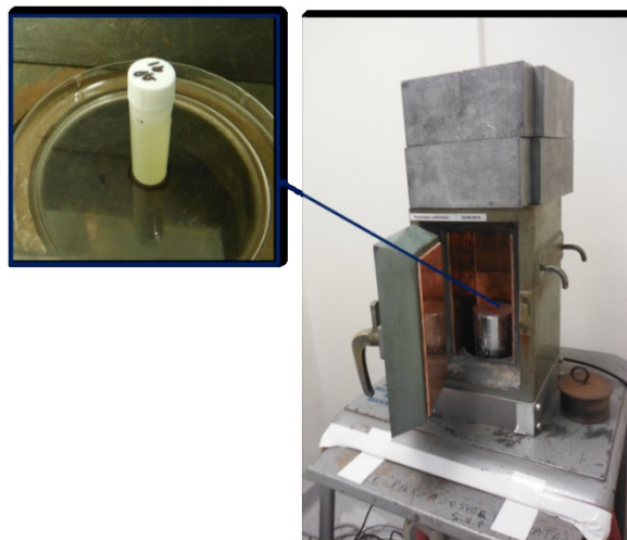
Figure 53 Picture the HPGe detector involved in the \gamma -spectrometry measurements of our samples.
