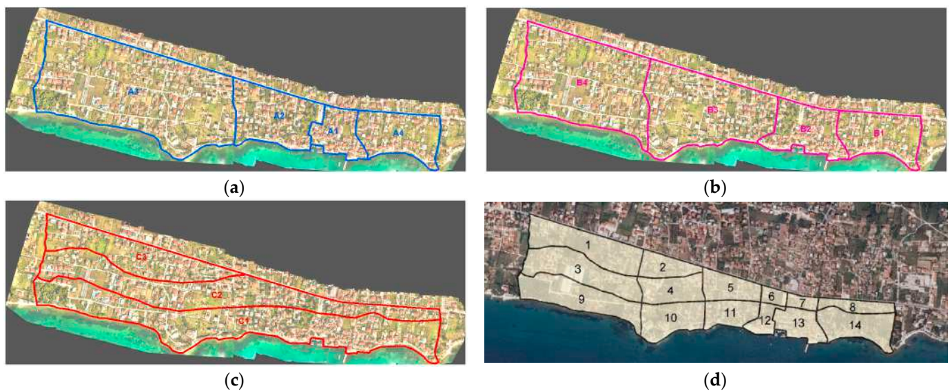
Figure 9. The creation of homogenous zones: (a) four areas defined by specific urban characteristics; (b) four areas defined by main roads; (c) three areas defined by terrain (contours 5 and 10 m); (d) intersection of layers resulted with 15 homogenous zones.
