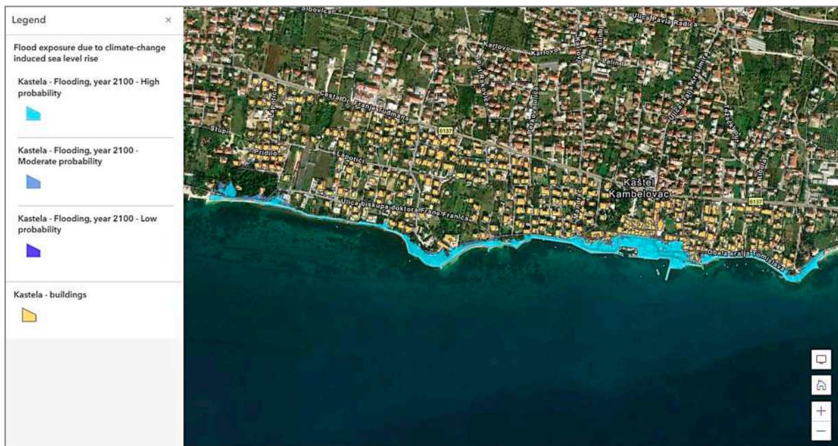
Figure 7. Distribution of critical zones most prone to flood due to impact of climate changes on sea level rise: scenario for year 2100.
