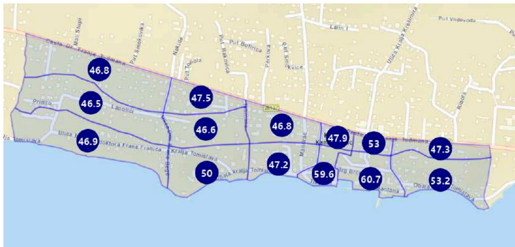
Figure 20. Results of the risk analysis for seismic, flood and extreme waves hazards for Level 1 (Scenario S-F-EW L1).
