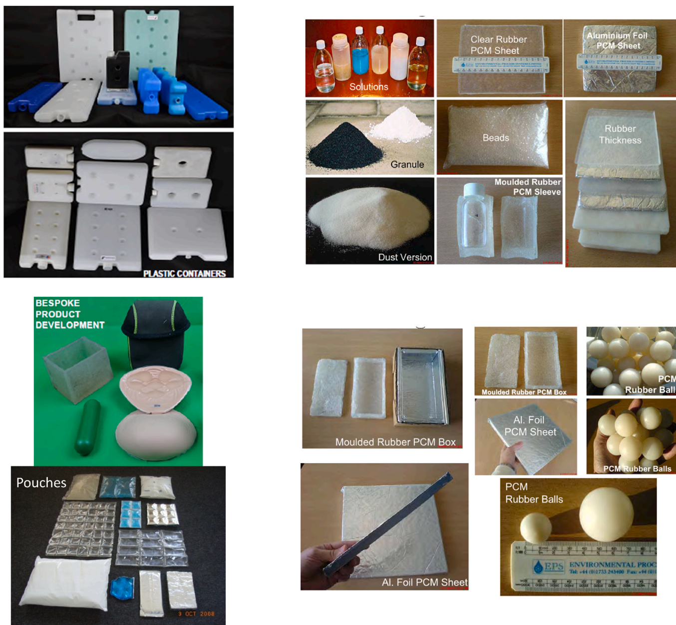
Fig. 7. PCM encapsulation examples [38].
