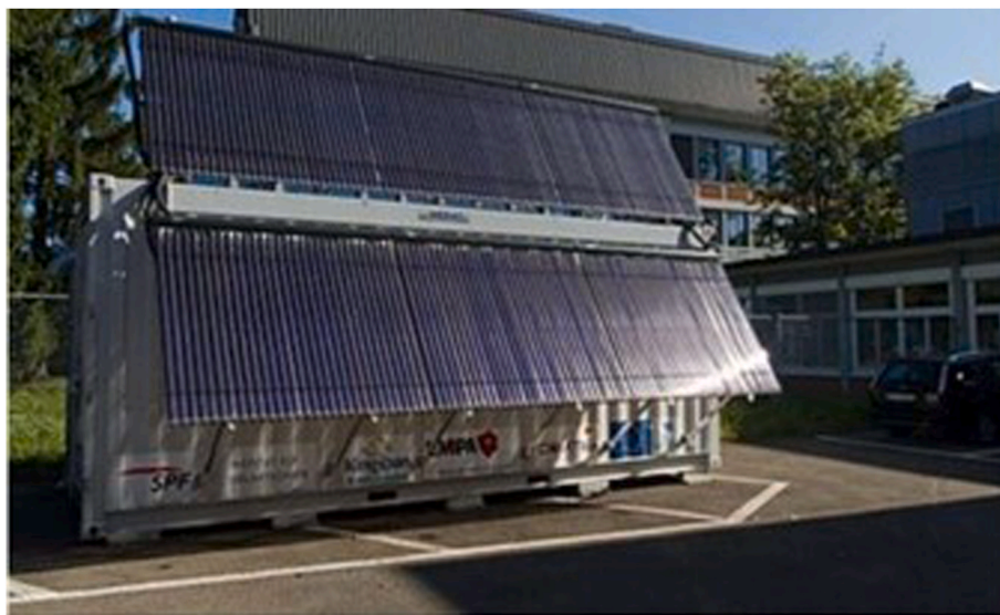
Fig. 41. Pilot-scale storage plant combining long-term sorption storage and short-term sensible designed to cover yearly energy demand of a low-energy single family home. Reprinted from B. Fumey, R. Weber, P. Gantenbein, X. Daguinet-Frick, Sascha Stoller, Reto Fricker, V. Dorer, "Operation Results of a Closed Sorption Heat Storage Prototype", Energy Procedia, Volume 73, Page 7, Copyright (2015), with permission from Elsevier.
