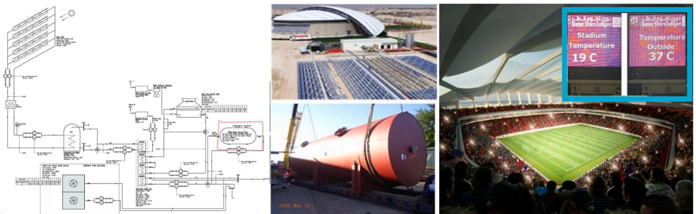
Fig. 25. Solar large scale off-grid cooling application in Qatar [101].
