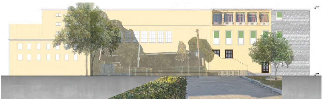
Figure 146. Survey of the main façade through forogrammetry; sketching of marble panels; and extraction of the complete model of the southern façade after filling in the missing parts
