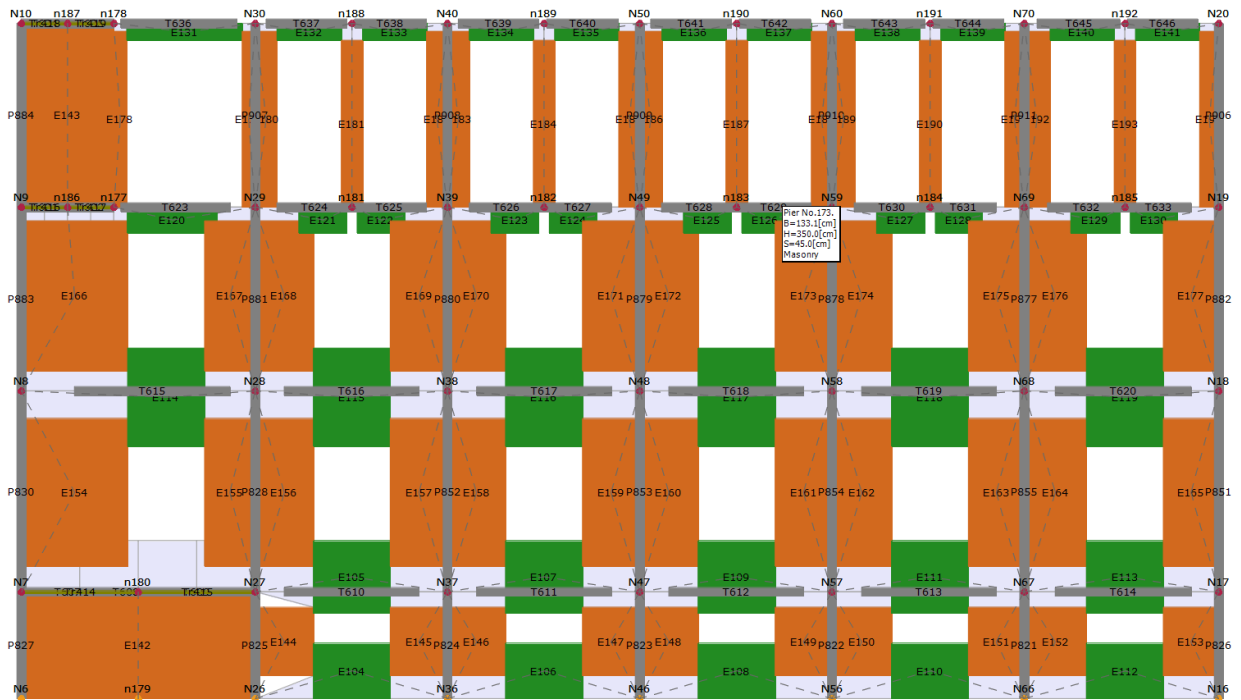
Figure 131. Numerical model of the main facade processed in 3Muri software
