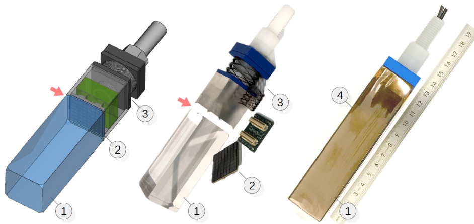
Figure 3.4: A design and construction sketch and disassembly photos for a LYSO crystal detector, with colour to show the major components. The LYSO crystal’s corners are chamfered to create a stable mount against the aluminium housing that holds the SiPM, as indicated by the red arrows. The labels stand for: (1) LYSO crystal; (2) SiPM array (88); (3) housing and mechanical system; (4) wrapping with three layers: Teflon as a reflector, Tedlar for light tightness, and Kapton [60] for mechanical stability.
