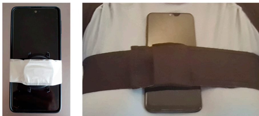
Figure 10. Setup of the reliability test during forward inclination. The SW Mobvoi TicWatch E2 and the smart harness developed together were compared to the gold standard system (smartphone with MATLAB mobile platform).
