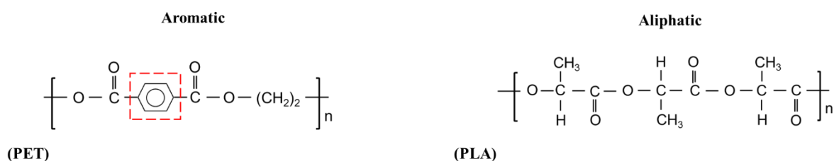
Figure 2.7: Comparison between representative aromatic and aliphatic polyesters, the benzene ring is highlighted in red
