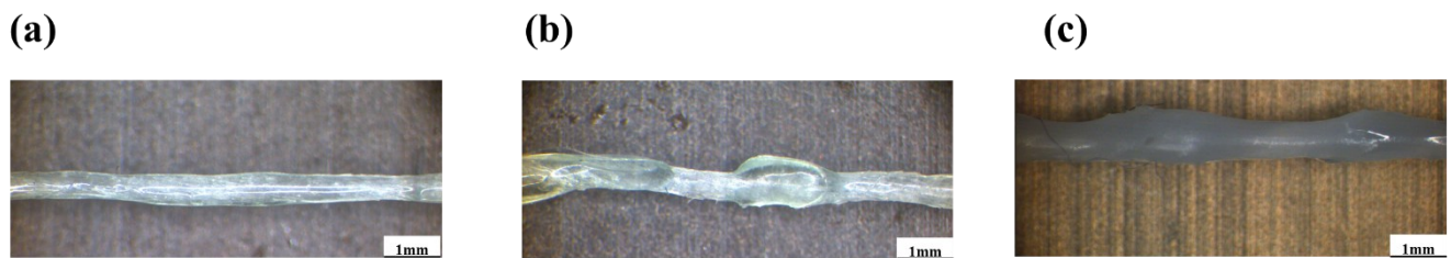
Figure 7.12: Preliminary analysis on dripping effect made with a) “Plant”, b) “Fast” and c) “Rigid” resin
