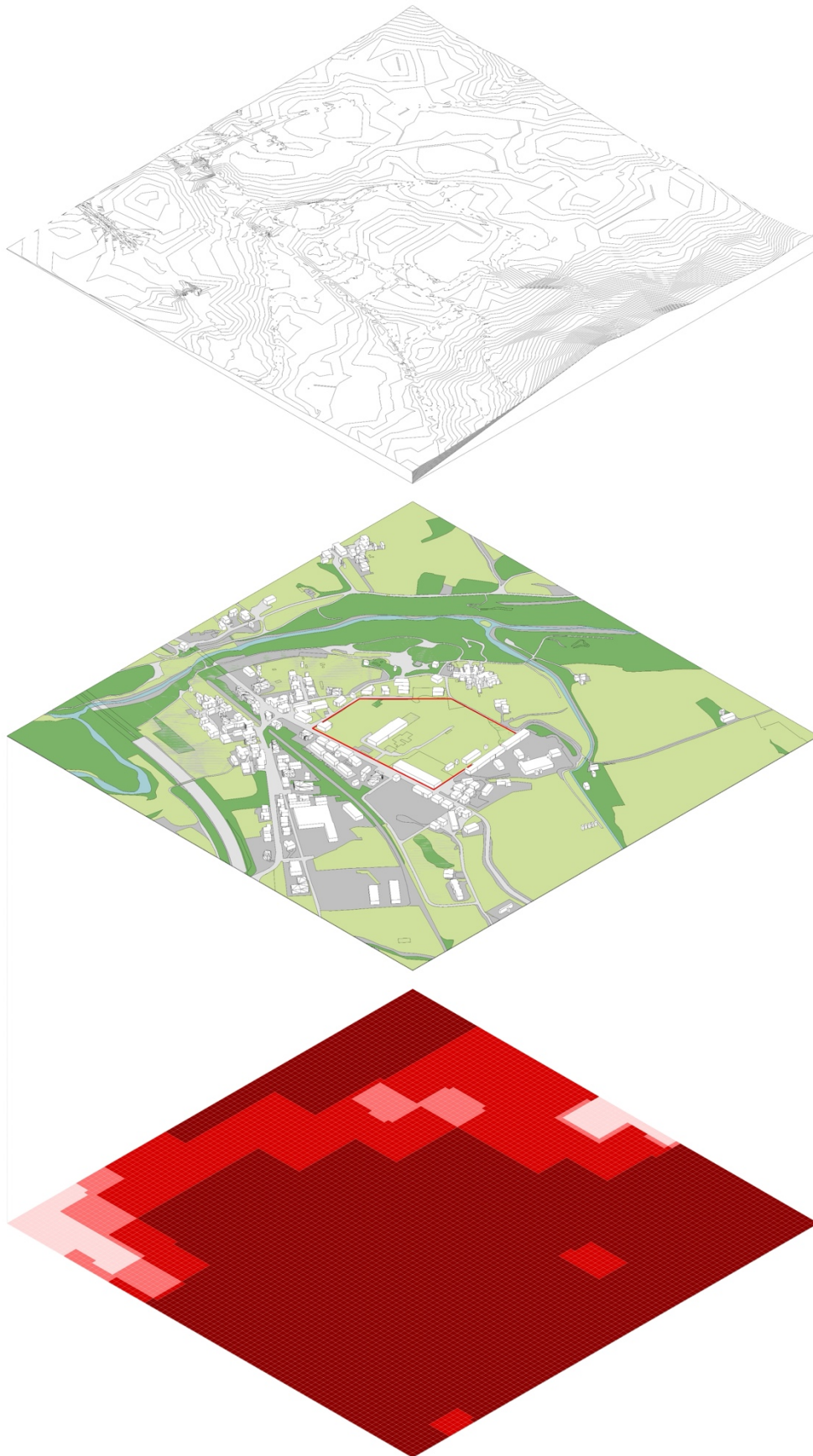
Figure 4.11 - Exploded axonometric view within Revit, showing the hierarchical composition of the Micro scale digital model: from the EO analysis layer (UHI represented) to land use, topography and project area
