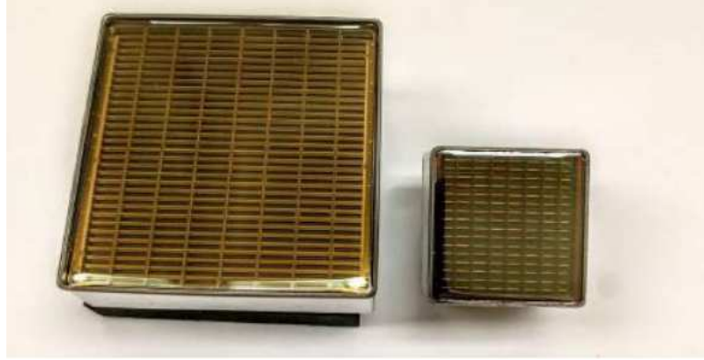
Figure 5.2: The MaPMTs selected for the upgraded RICH detectors with the 2-inch model on the left and the 1-inch model on the right.
