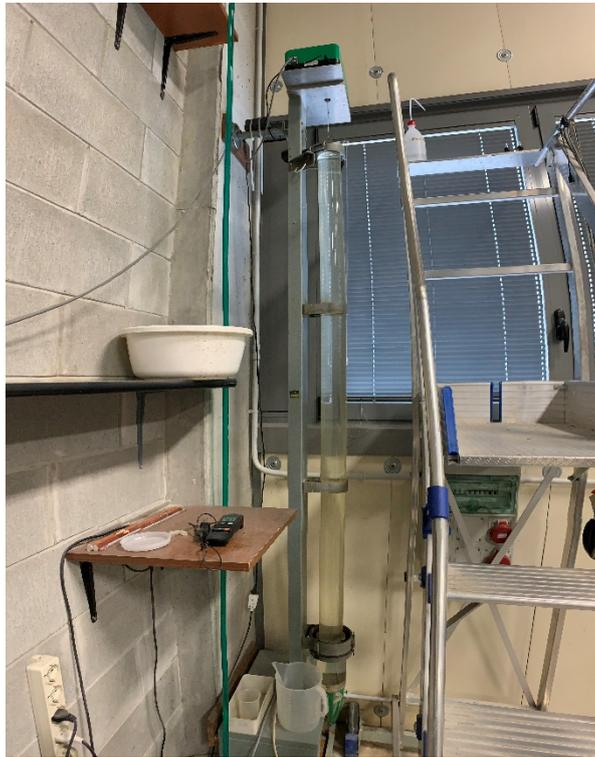
*Figure 4-16: Sedimentation balance Physics and Earth Sciences Department at University of Ferrara (ITALY)*
