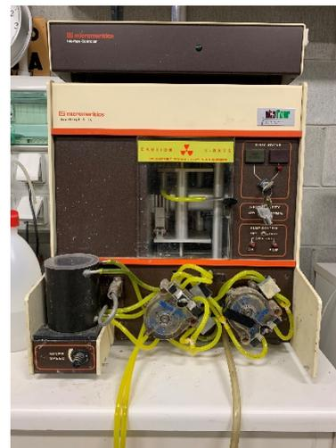
Figure 4-18: Left) Simplified schematic diagram of the X-ray Sedigraph instrument (Syvitski, 1991); Right) Micromeritics Sedigraph 5100 at Physics and Earth Sciences Department at University of Ferrara (ITALY).
