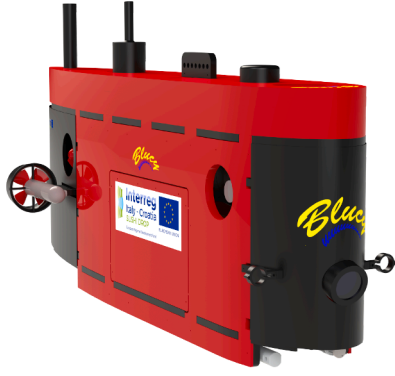
Fig. 3. Blucy underwater vehicle with 6-thruster configuration.
