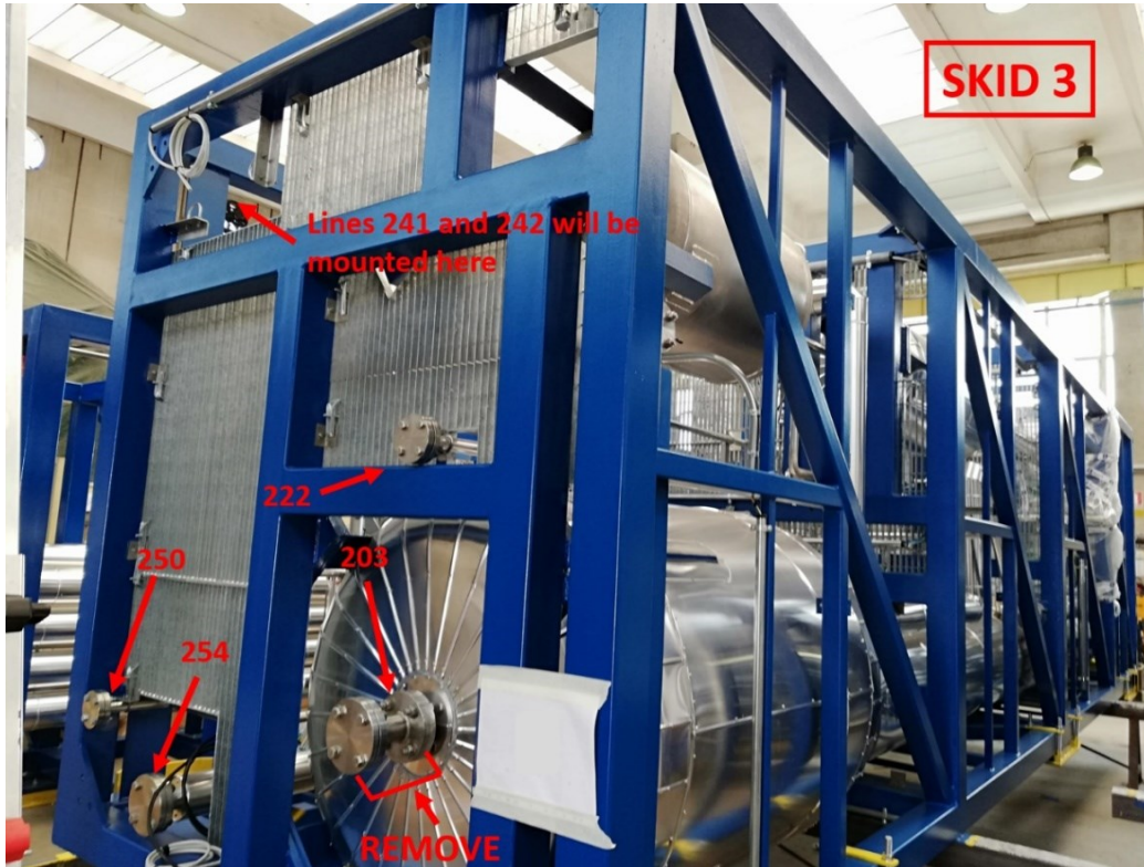
Figure 57: Blind flanges of skid 3 to be removed before the installation of skid 3 on skid 1.
