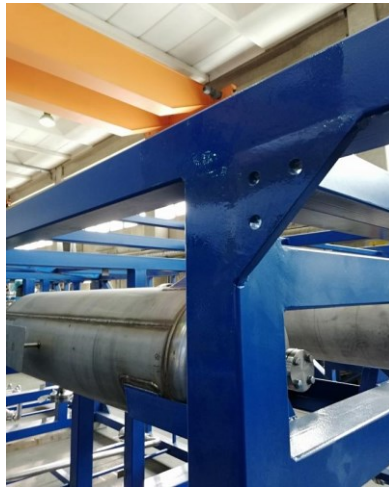
Figure 46: Triangular plates for the skid fixing
