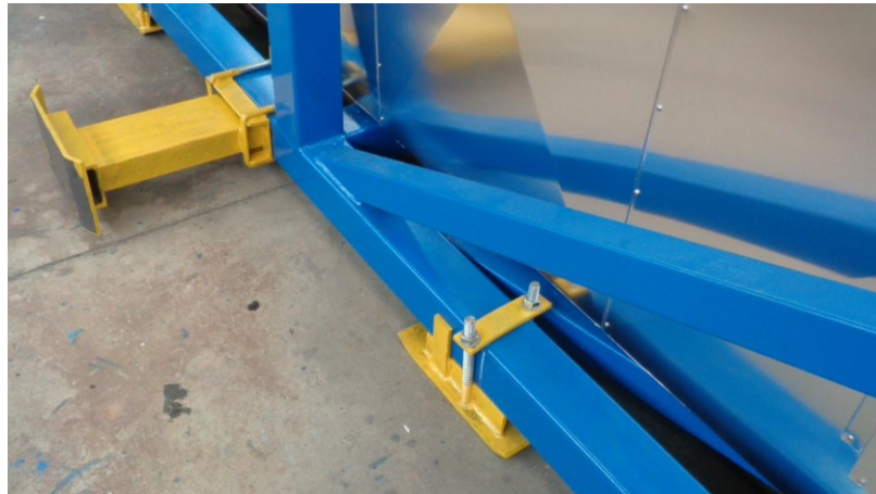
Figure 45: Temporary yellow slides, provided on skid and tanks. They shall be removed before positioning operations into the laboratory hall.
