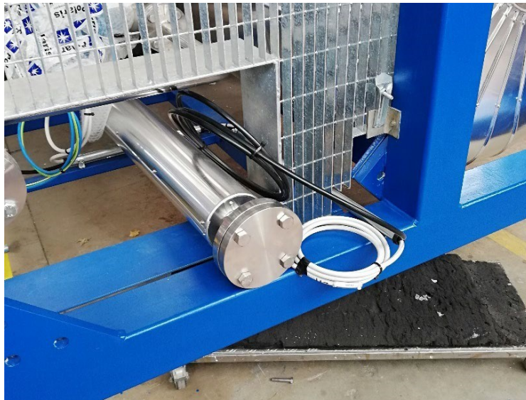
Figure 7: Interconnecting pipeline sealed with a protective blind flange
