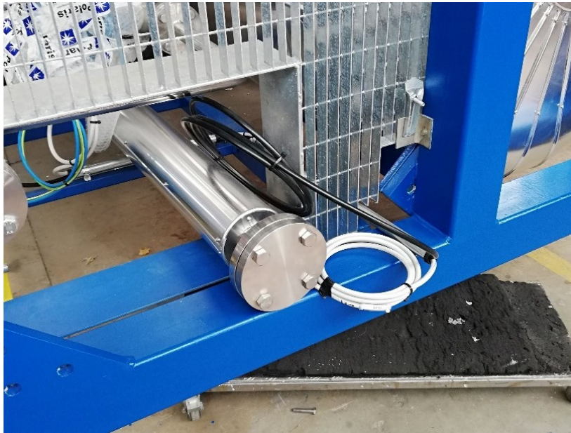
Figure 52: Interconnecting pipe sealed with a protective blind flange
