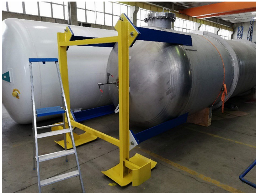
Figure 4: temporary yellow slides, provided on skid and tanks. They shall be removed before positioning operations into the laboratory hall
