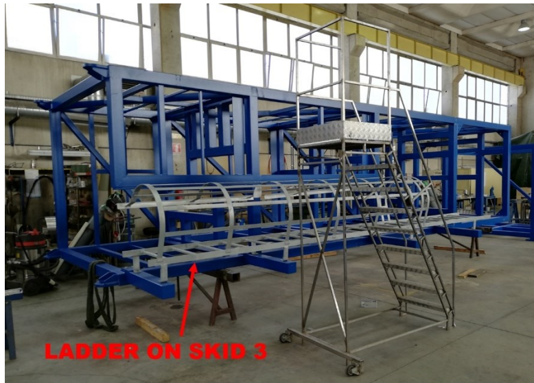
Figure 55: Position of the vertical ladder on skid 3
