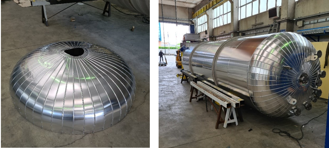
Figure 75: Tank insulation with Rockwool and a protective layer of aluminium. On left, some details of the aluminium protective layer properly shaped to fit the tank dome.
