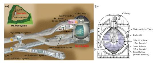
**Figure 7 - (a)** KamLAND experimental site and **(b)** the schematic design of the detector. **(a)** There are 2 types of liquid scintillator purification system (liquid-liquid extraction and distillation). The water purification is operated to produce pure water filled in the OD. **(b)** The shaded region in the LS shows the fiducial volume for  $\bar{v}_e$  in Period 3.
