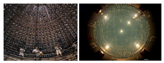
Figure 13 – a) The scaffolding, cleaned in the entrance clean room, in uninstallation phase. b) A picture of Borexino taken from cameras mounted inside the SSS.
