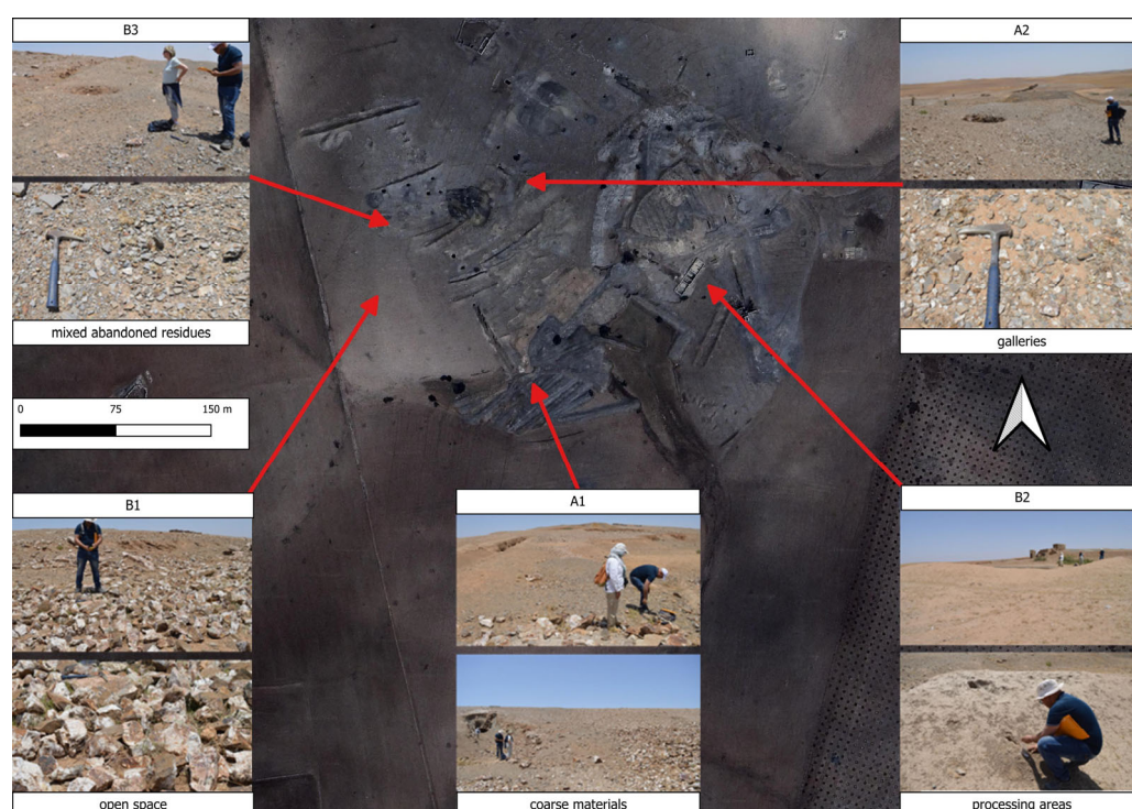
Figure 10. The spatial distribution of mining residues identifying different zones (red arrows) with varying mineralogical compositions in the Sidi Bou Azzouz abandoned mine (Google Earth Pro-Image © Airbus 2025, acquired on 2 February 2022).
