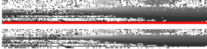
Figure 49: Below, a polar grid map of the RADIATE dataset before calibration. The white band at the top is due to the point cloud being cropped. Above, the same polar grid map after calibration.
