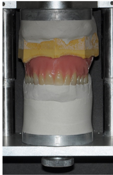
Figure 2. Denture model placed on the verticator using plaster keys.
