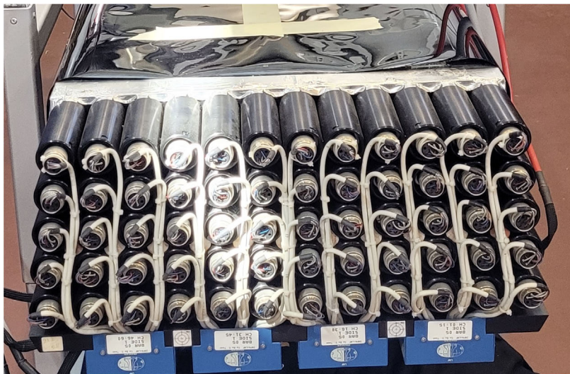
Figure 3.4: View of one end side of an ECal barrel module showing the array of photomultiplier tubes. Photo from [93].
