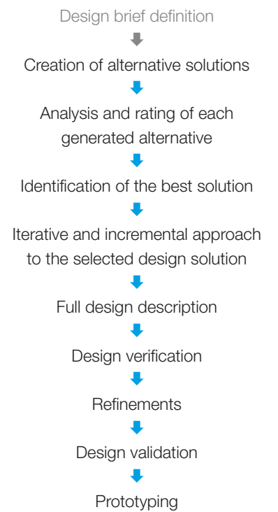
Flow diagram describing the Design Solution Definition process adopted in this research to achieve the first prototype
