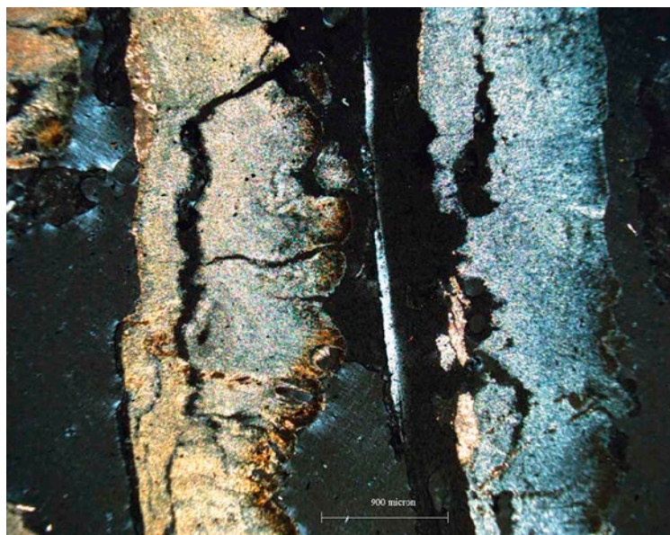
Figure 5a. Sample TOR2bis: microphotograph showing the high porosity of the oxalate patina (cross polarized light).
