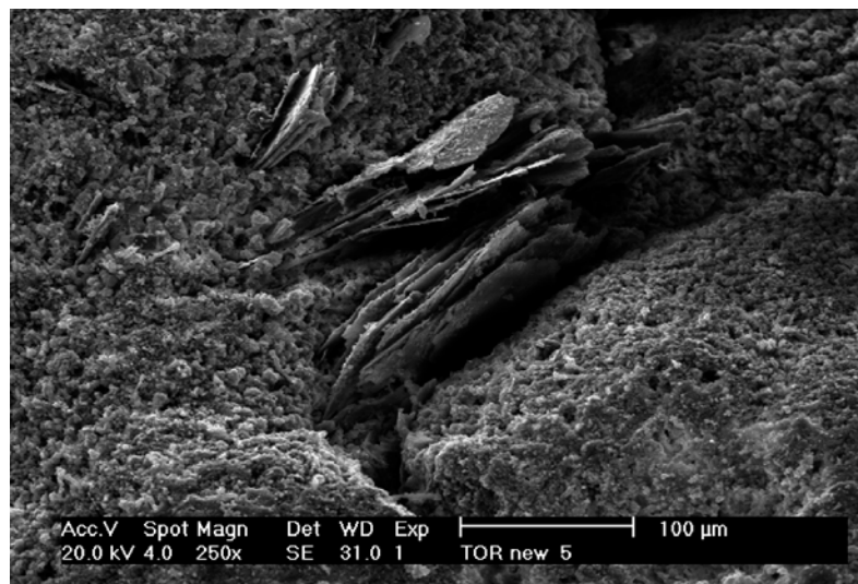
Figure 8a. SEM microphotograph of sample TORNEW5 showing a pair of muscovite crystals.
