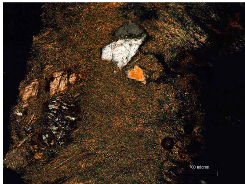
Figure 6b - Sample TOR4bis: microphotograph highlighting the presence of quartz crystals (white-yellow color) and calcite (pink color, on left) (cross polarized light).
