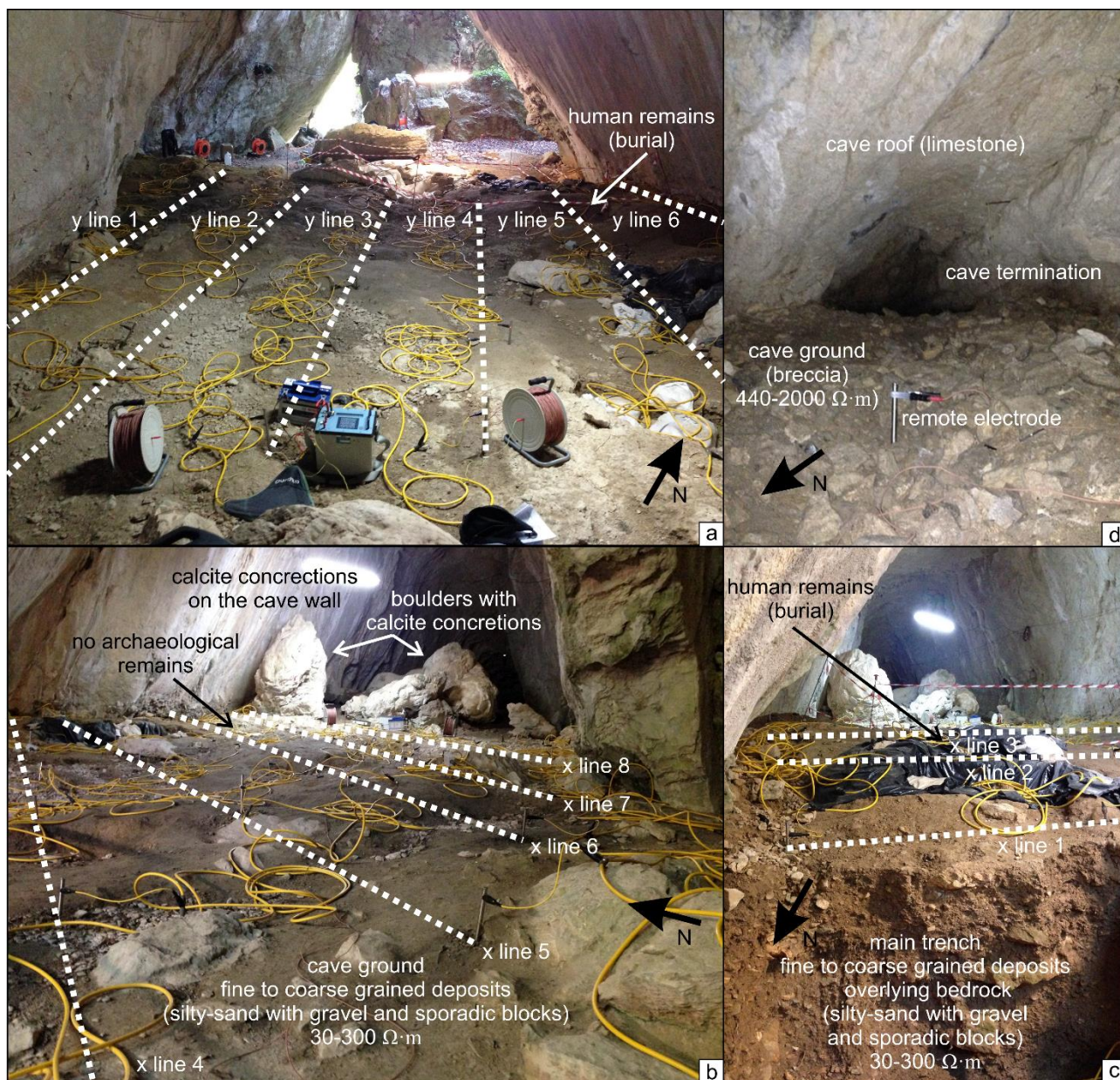
Fig. 4: Pictures showing different views of the 3D ERT survey grid along with lithological description.
