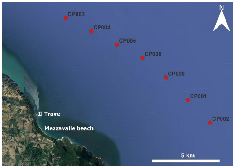
Figure 24: Coastal points defined in front of the area of interest. The points are positioned on the 20 m depth contour of the bathymetric dataset provided by ARPAE.
