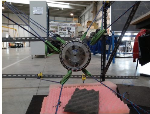
Figure 4. Experimental set up for estimation of rigid body inertia properties
