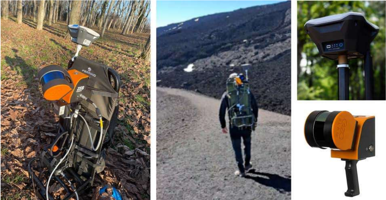
Figure 3 Custom backpack-mounted configuration used for the GeoSLAM ZEB Horizon handheld LiDAR survey. The metallic frame was adapted to host the scanner, the data logging unit, and the Emlid Reach RS+ GNSS antenna (operating in RTK mode), allowing autonomous data collection and accurate georeferencing of the point cloud. The system enabled the operator to perform extended surveys efficiently, even across large areas, as shown in the central panel. The right panels show details of the GeoSLAM ZEB Horizon unit and the Emlid Reach RS+ GNSS antenna.
