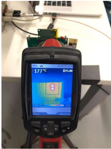
(a) Picture of the thermal camera measuring the directly polarized SiPM. The sensor can reach more than 175^{\circ}\text{C} , but has not to overcome the value of 180^{\circ}\text{C} .
