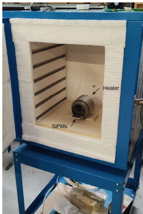
Figure 4.9: The oven used to perform the first annealing in the laboratory of INFN Ferrara.
