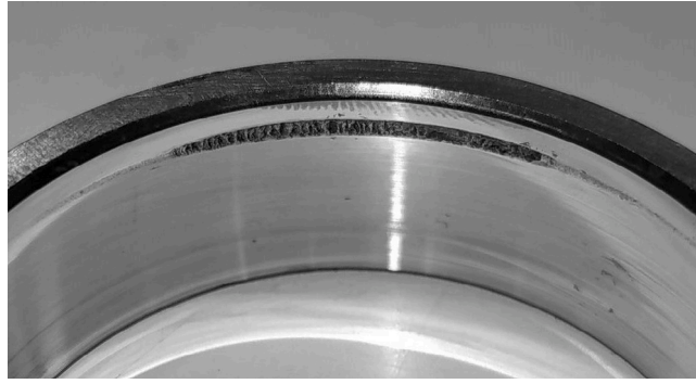
Fig. 10. Extended defect on bearing outer race at the end of test E1.
