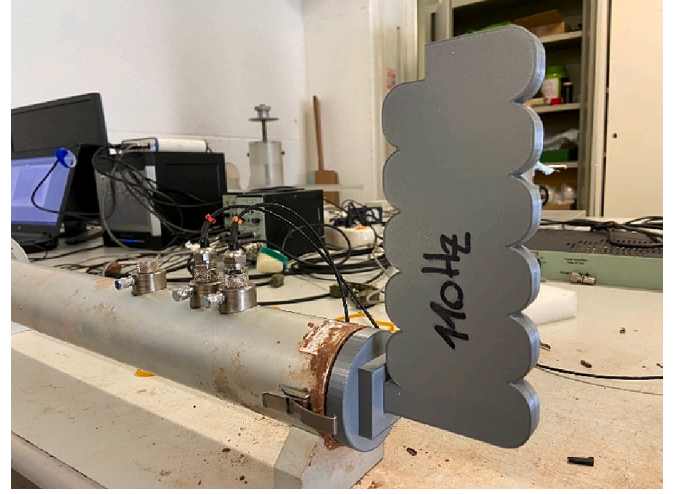
Fig. 4. Normal incidence sound absorption coefficient – experimental measurement setup according to standard.
