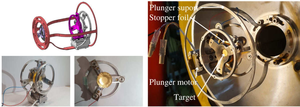
Figure 3.9: (Top left) CAD drawing of the plunger device. Figure taken from Ref. [75]. (Bottom left and right panel) Pictures of the target and the holding structure of the plunger device installed in the reaction chamber of GALILEO.
