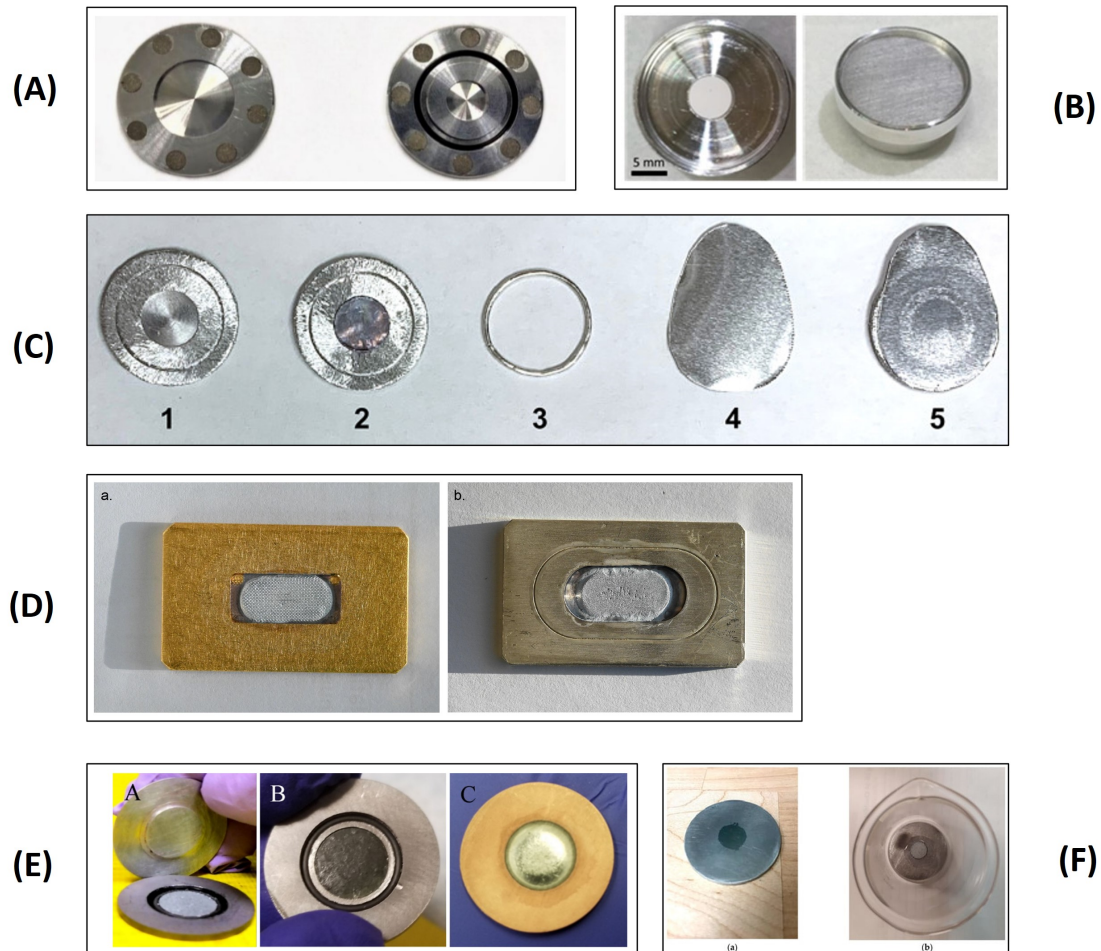
Figure 1.8: Different targets design, produced by different groups: (A) Capsule design, using powder pellets [25]; (B) Pressed CaO target (6 mm × 0.5 mm) in Al capsule for ^{44}\text{Sc} [26]; (C) ^{nat}\text{Tl} Target assembly for ^{203}\text{Pb} production [27]; (D) Electrodeposited ^{70}\text{Zn} targets from fresh and recycled electrolyte [28]; (E) Different Cr targets on the Cu backing for ^{52}\text{Mn} production [29]; (F) Fused Zn target for ^{68}\text{Ga} production [30].
