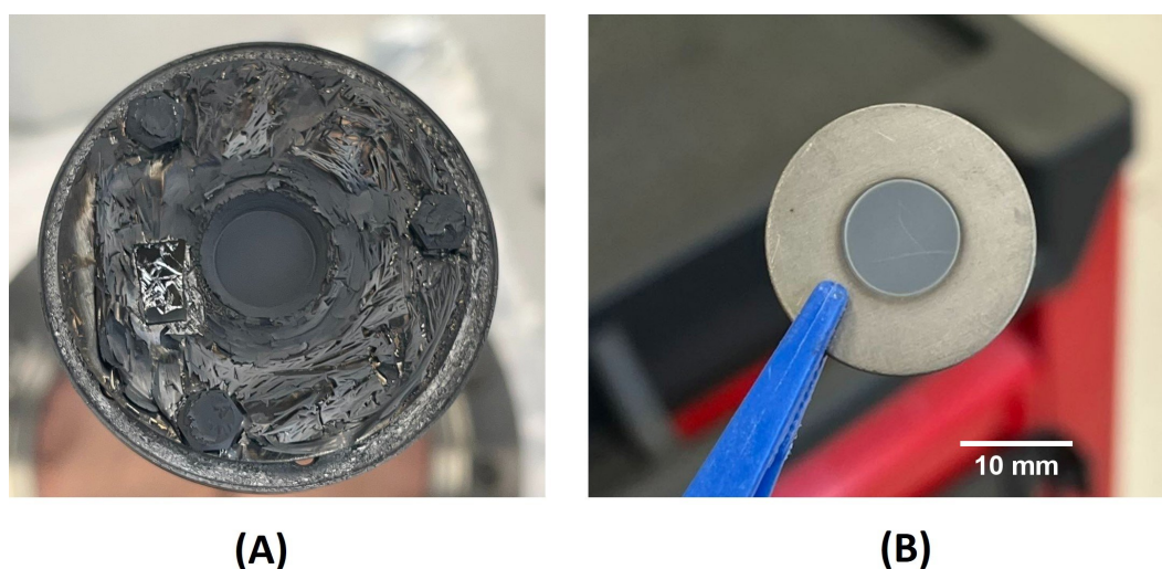
Figure 5.14: Deposition results of Cr-8 test: picture of sample holder after the deposition (A) and manufactured target (B).
