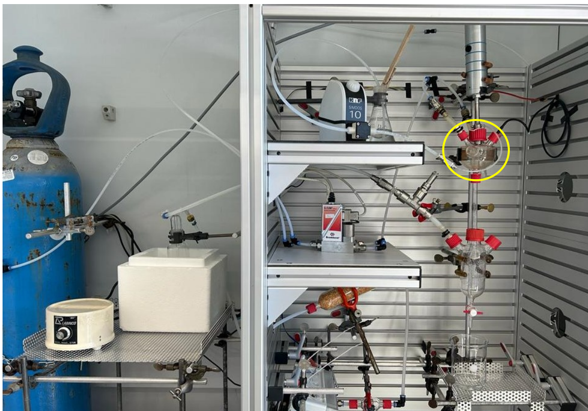
Figure 30 Experimental set-up with 56 mL aerosol chamber (yellow circle).
