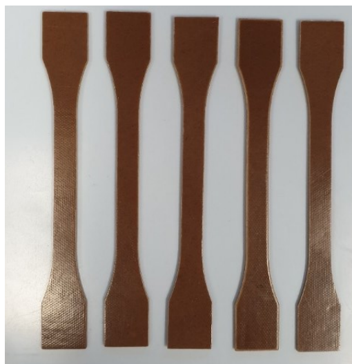
Figure 39. Compression molded specimens of PLA filled with wood
