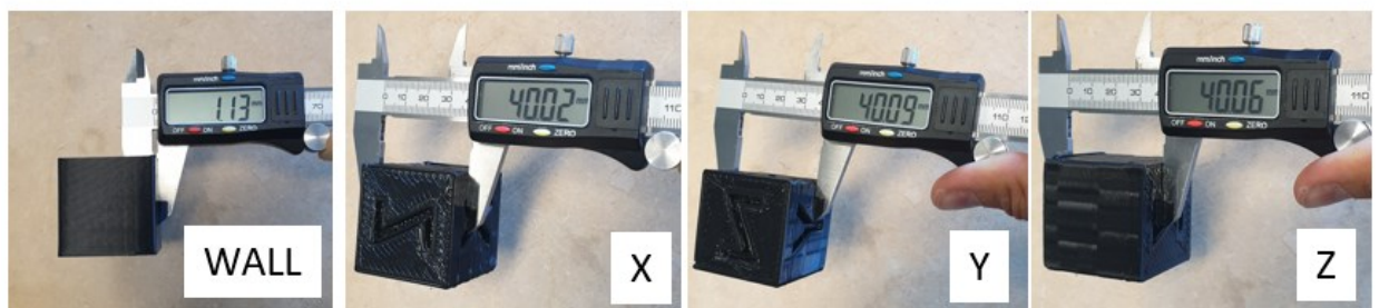
Figure 17. Measurements of bead width and cube along directions x,y, and z
