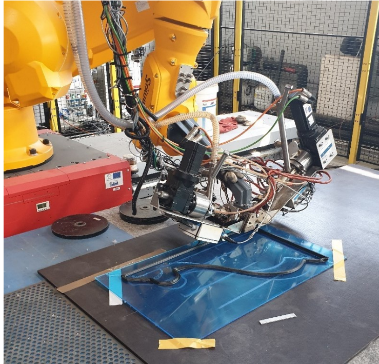
Figure 20. 3D pellet extruder robot arm during printing
