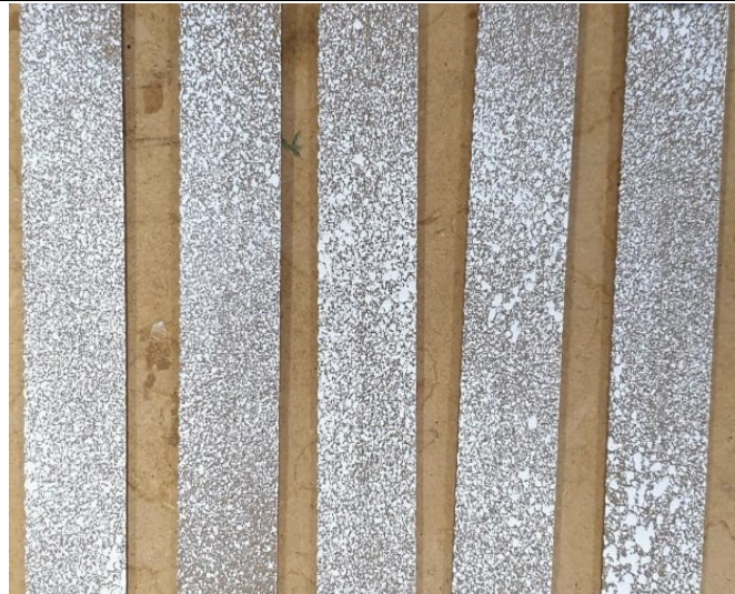
Figure 33. Samples painted for DIC acquisition
