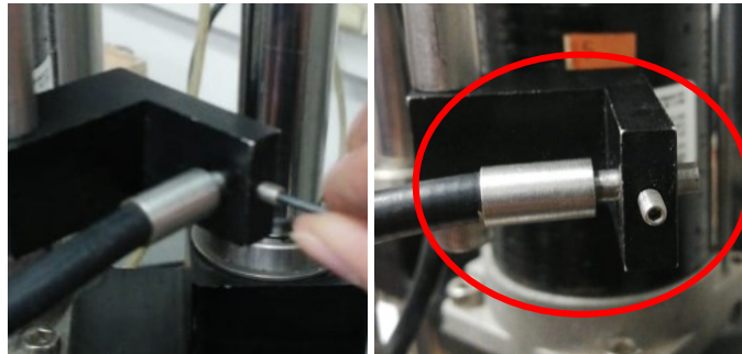
Figure 128. Place and adjusting the laser.
