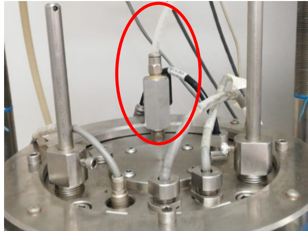
Figure 132. Connect to the confinement of the chamber.
