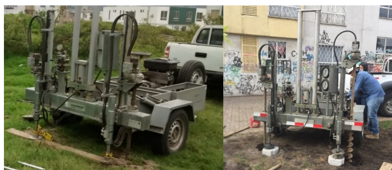
Figure 33. CPT Test being performed in the South of Quito
