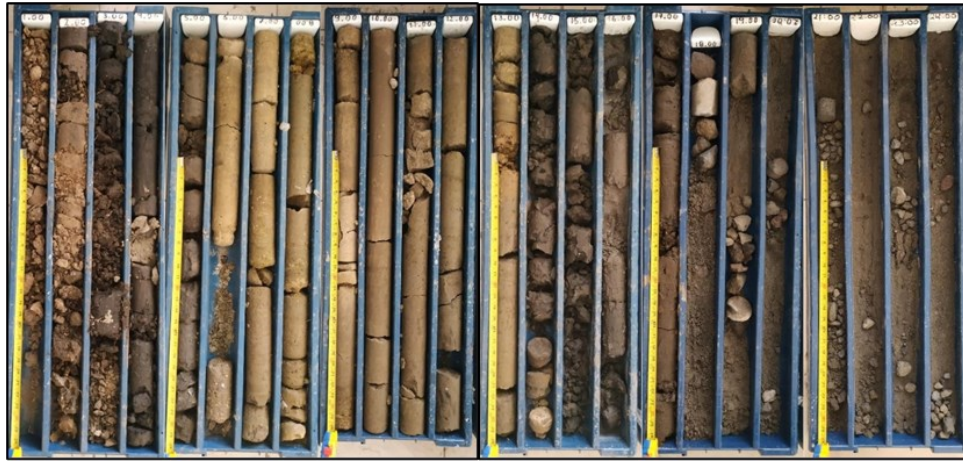
Figure 44. Example of the continuous sampling in Borehole 14, applied to the 21 sites.
