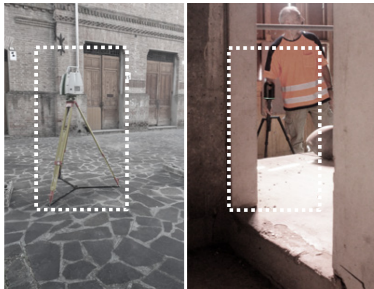
Fig. 93. The Laser scanner survey campaign was carried out in September 2020 using Leica C10 and Leica BLK 360 laser. Developed by M. Suppa
