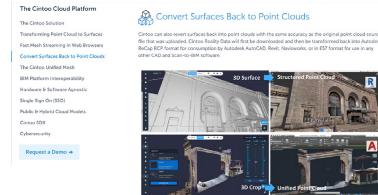
Fig. 109 - CINTOO platform transforms massive laser scanning data into a format compatible with the cloud and BIM. The data can be shared, visualised, measured or used in Scan to BIM workflows. Image from https://cintoo.com/
