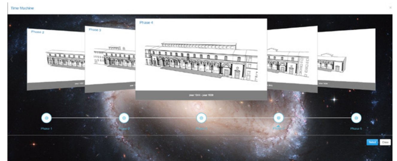
Fig. 112 - The image shows the time machine function of inception that allows visualisation of the model by historical steps. Developed by INCEPTION team http://www.inceptionhbim.eu/platform .
