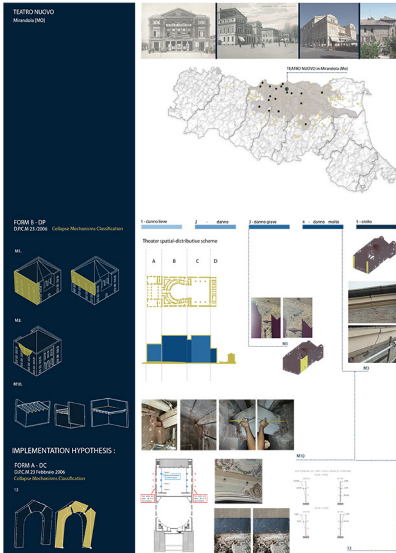
Fig. 53 The damaged form applied for the Theatre of Mirandola's seismic damage survey, the card's fields from the study of specialistic investigations, do not damage the proscenium arch and the plafond. The hypothesis of implementing the B -D.P. sheet with the A-DC sheet with which the collapse mechanisms related to the picturesque arch and the palfond can be described. Developed by M. Suppa
