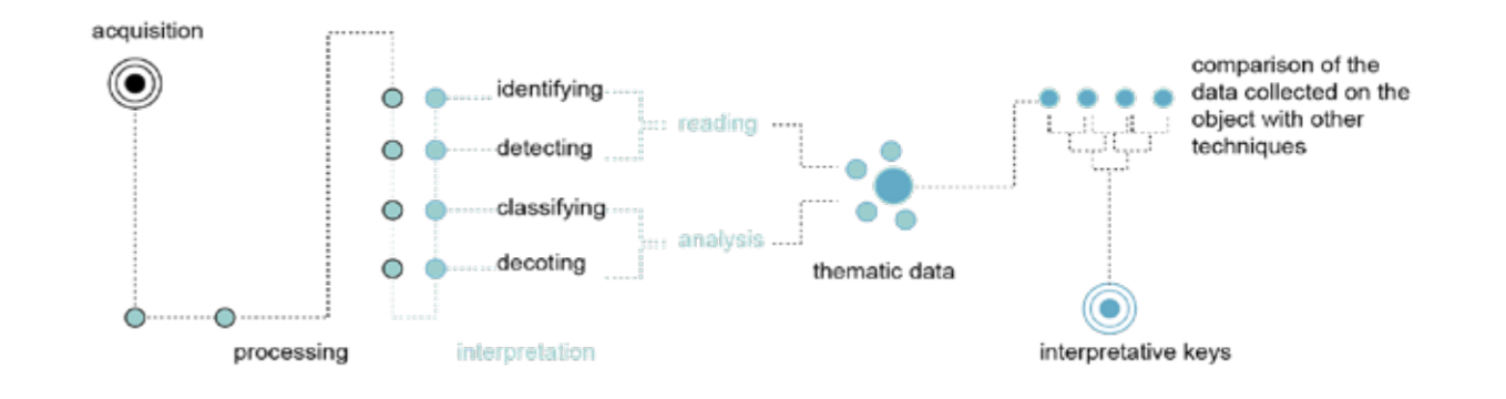
Fig. 97 Methodological diagram of the interpretative analysis of the point cloud to draw the map of surface degradation. Developed by M. Suppa
