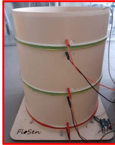
Figure 5-15: The mock-up of the photobioreactor, with the coils placed at a z = 0 \text{ mm} (bottom coil), z = 200 \text{ mm} (middle coil), z = 402 \text{ mm} (upper coil).
