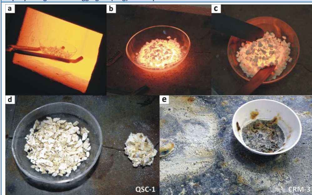
Fig. 2.7: Overburning Test (OT) method. Extraction and evaluation procedures. a = sample extraction after 3 h burning at 1300 °C. b = fast cooling. c = block extraction. d = visual evaluation and block weighing. e = example of a fused sample (CRM-3).
