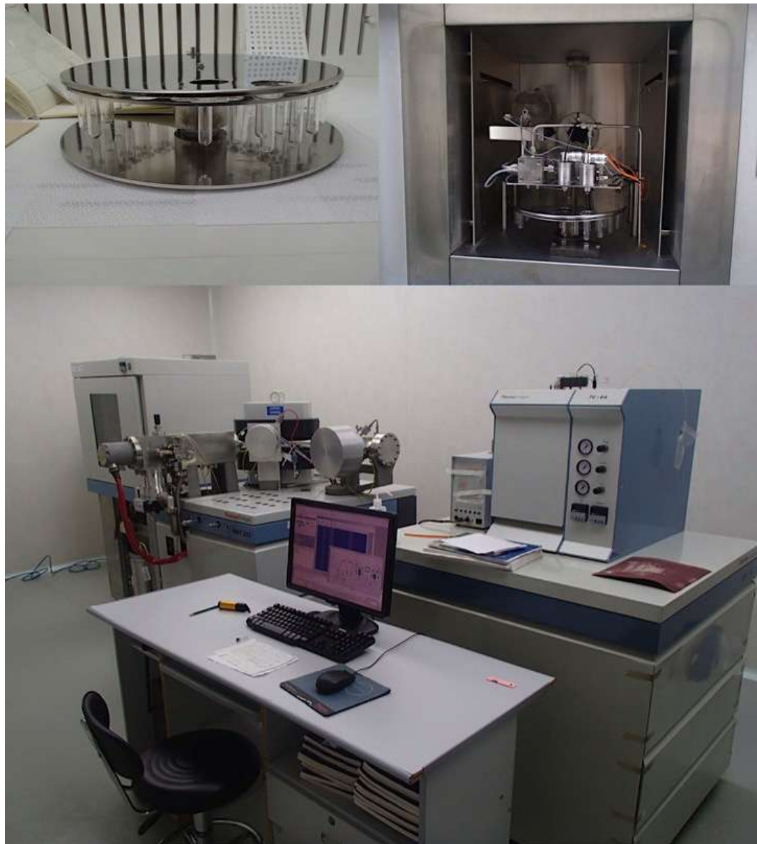
Figure 34. One of the on-line automated carbonate preparation system (Kiel Carbonate Device) linked to Finnigan MAT-253 mass spectrometer at the Isotope Laboratory of School of Geographical Sciences at the Nanjing Normal University. © MGPGFaylona July 2017
