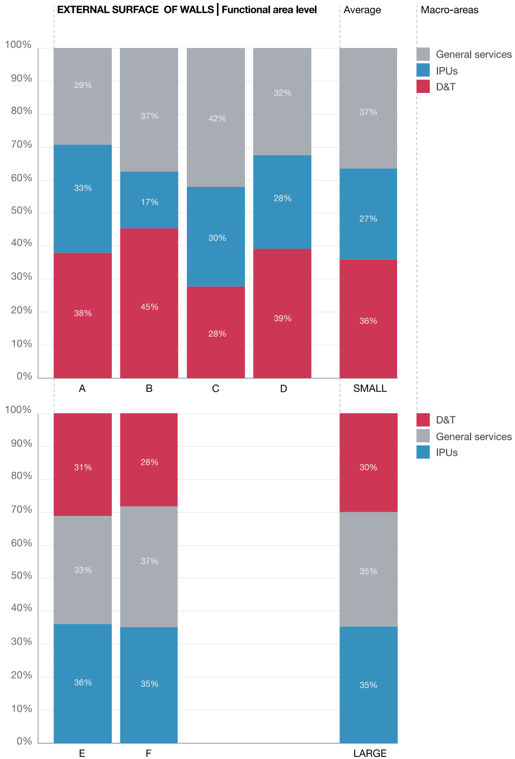
Figure 3.11. Distribution of external surface of external walls by macro-area on the base of functional area level distinction
