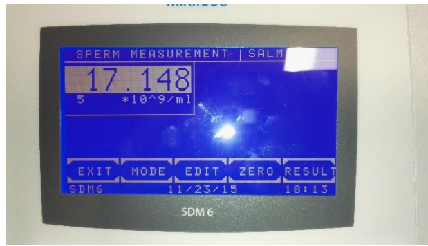
Figure 25: picture of the photometer SDM6 (by Minitüb GmbH and Cryogenetics®) showing the data output. In the example the measurement of the milt concentration is 17,148 \cdot 10^9 /ml.
