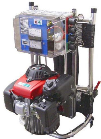
Figure 5: a) ichthyologists sampling by electrofishing with backpack model electrofisher b) EnginePowered Electrofisher ELT6011, 300/500V Max, 1300W, Honda engine, Han-grass, Germany
