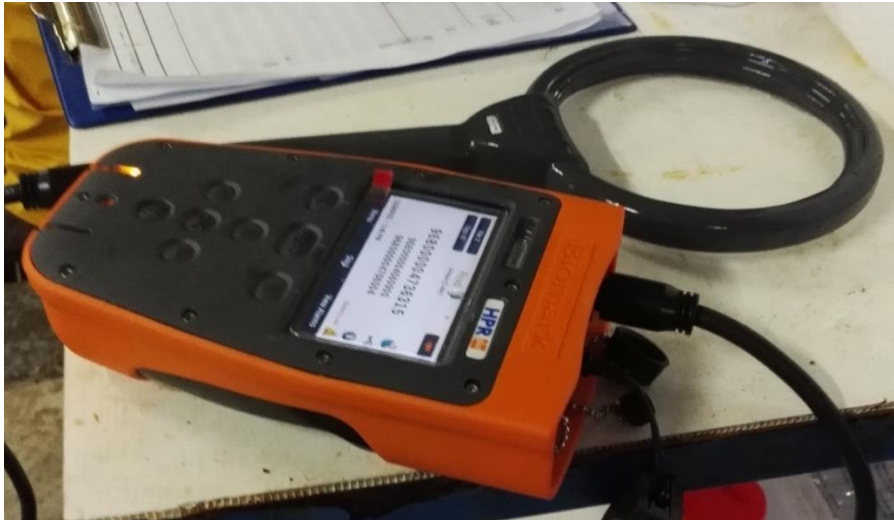
Figure 6: Biomark HPR Plus™ reader used in Centro Ittico Valdastico (VI) to read PIT-tag barcodes of the marble trout breeders.
